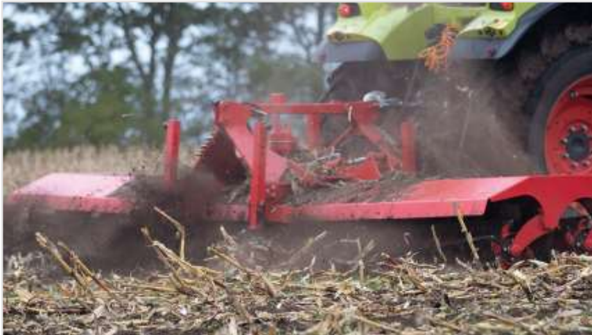
Three-point linkage on Top-Cutter Solo, enabling both front- and rear mounting
