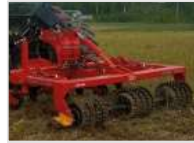
2.50 m with hydr. release system and asynchronous Star roller.
