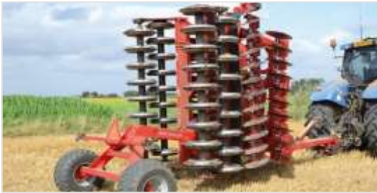
5.50 m Disc-Roller Contour with Twin V-Profile roller and material
