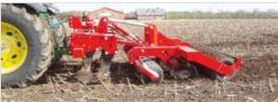
Combi-Disc with the tines lifted free from the soil, meaning that only the Disc-Roller's function is in
