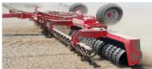
6.30 m Tip-Roller with Cambridge rings and Spring-Board with Ø16 mm longfinger tines
