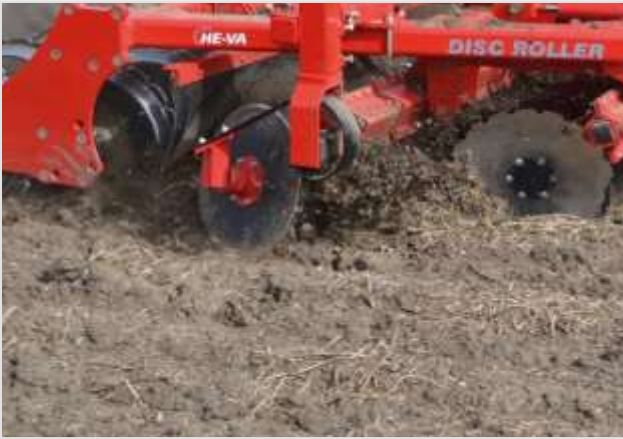
Standard equipment on all models: Adjustable edge disc for retain soil on right side.
