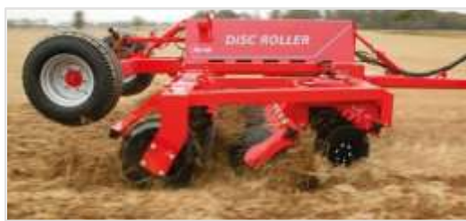
5.00 m with V-Profile ring and material damper
