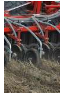
Seeding with disc coulters with 75 mm wide depth/ press wheel. 1 row placed in centre line of the tine, after packer roller.
