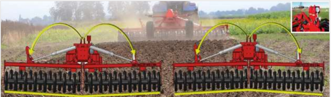
Standard equipment on models with 2 and 3 section: HE-VA SAT-System: Hydr. adjustable weight transfer system, ensuring equal weight transfer in the total working width, resulting in the fact that the wing sections follow the terrain.
