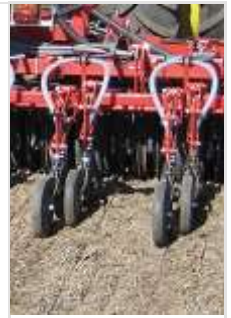
Seeding with disc coulters with 75 mm wide depth/press wheel. Placed in 2 rows around centre line of the tine, after packer roller.
