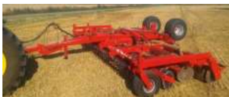
5.50 m Disc-Roller Contour with Twin V-Profile roller and material damper guard.
