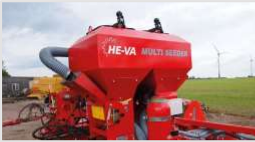
Multi-Seeder Twin 2x100-8-HY-AC 593 x 926 (1,180) mm H=935 (1,075) mm
