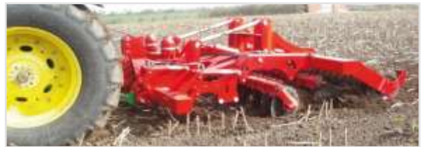
Combi-Disc with the tines in max. working depth, ensuring a soil loosening, cultivation and a consolidation.
