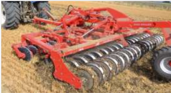
5.50 m Disc-Roller Contour with Twin V-Profile roller and material
