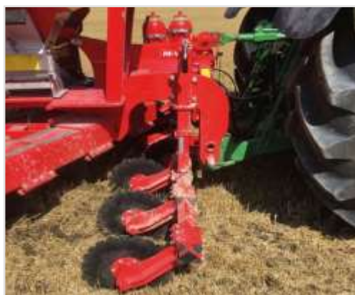
Frame for roller coulters with roller coulters Ø470
