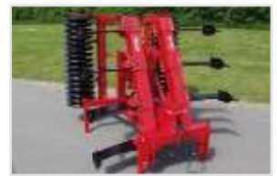
4.00 m with hydr. fold., 7 tines, V-profileroller and Quick-Push stone protection.
